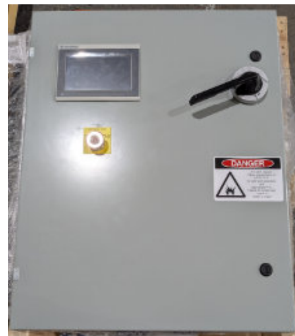
CMAXX integrated control panel (ICP) example. The ICP contains a 480 V AC input circuit breaker, 480 V AC terminals for the CMAXX fan (1), terminals for the cleaning solenoid control wiring (2) from the timer control board (3), terminals for remote interlock monitoring (5) and accessory wiring (6) and tubing inlets for the filter differential pressure sensors.
