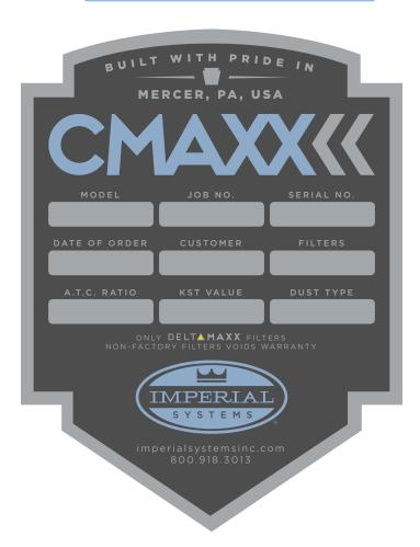
**Model** – Model of dust collector that you have. The number in the model name represents the quantity of filters in the unit.
