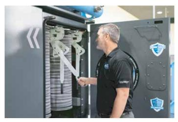
2. Using lever in extended position, lower lift rail assembly. Repeat on both sides of the filter before attempting to remove.
