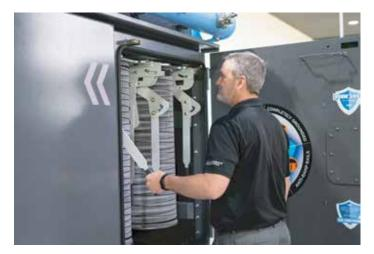
3. After lowering lift rails, remove the filters. Either grasp the filter by the metal pan on top, or use the filter tool. Only use the filter tool to capture the filter by the metal pan. Do not handle the filter media with your hands or the filter tool.
