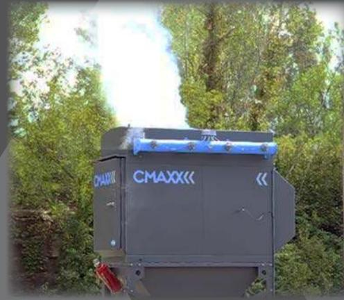
With cover on explosion vent, 100% of the flame front forced through the IDA DeltaMAXX Filters. No spark or flame present.
